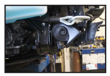
14. Align the holes in the side plate to the existing holes in the frame and loosely install the 3/8" hardware (white).
