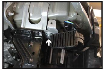
9. Using a 10MM socket, remove the screw from the PS horn and set the horn aside.
