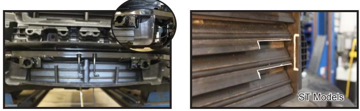
13. Hold the baseplate up to the vehicle and trim the plastic intake to allow the baseplate to be installed onto the frame.
