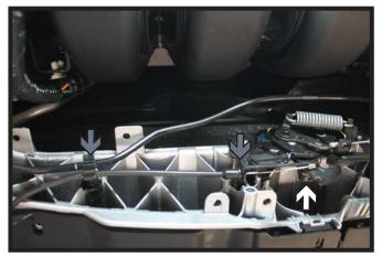
On the back side of the fascia, unhook the hood release cable from the latch (white) and unsnap the cable from the clips (gray).
