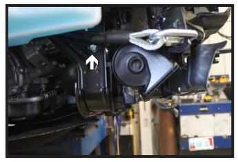
Reinstall the washer reservoir using the bracket on the baseplate and new hardware. Reinstall the horn to the lower existing hole (white).
