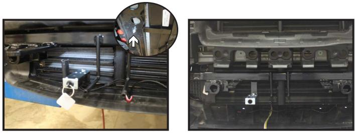
18. **Optional Breakaway (Baseplates with Serial# lower than 00045) :** Install the bracket to the existing hole in the crossmember (inset) with a 1/4" bolt and lock nut. Install the breakaway to the bracket with the supplied 1/4" hardware (Left).
