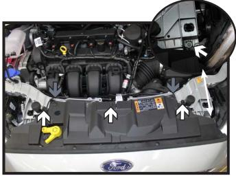
2. Using a T30 Torx, remove the five (5) screws from the top edge of the fascia (white). Remove the two (2) push pins from the outer edges (gray).
