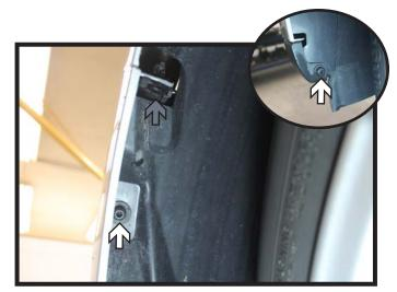
4. Using a T30 Torx, remove the two (2) screws from the edge of the wheel well (white). Also remove the push pin from the fascia/fender joint (gray). Do this on both sides of the vehicle.
