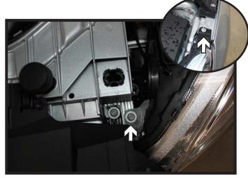
Using a T30 Torx, remove the two (2) screws from the headlight, disconnect and set aside. Do this on both sides of the vehicle.
