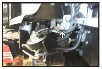
17. Bend back the webbing and reinstall the wheel well brace. Install the horn to the webbing's existing hole (white).
