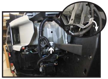
On the driver side, using an 8MM socket, remove the screw from the wheel well brace (white). Once the screw is removed, bend the webbing downward far enough for baseplate clearance (inset).
