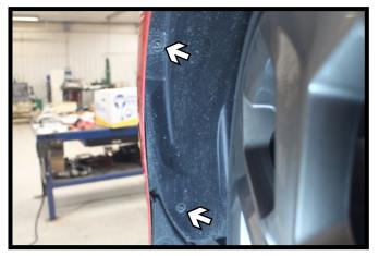
Using a T25 Torx, remove the two (2) screws from the wheel well. Do this on both sides of the vehicle.
