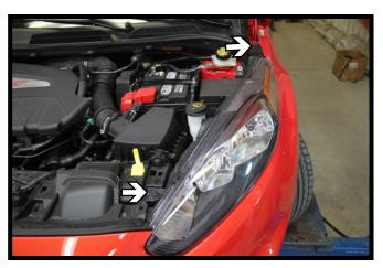
5. Using a T30 Torx, remove the two (2) screws from the headlight. Disconnect the electrical line and set the head light aside. Do this on both sides of the vehicle.
