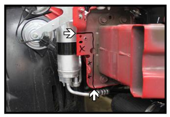
Trim the face of the frame extension just below the rib (top arrow) back to the face of the frame (bottom arrow). Do this on both sides of the vehicle.
