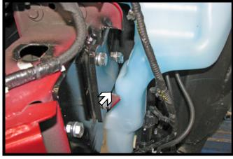
14. Reinstall the washer reservoir. Checking the clearance on the lower part of the reservoir making sure it is not rubbing on the baseplate. It should have minimum 1/16" clearance. If necessary pull the reservoir back and re-tighten the bolts. Reinstall the latch support brace.
