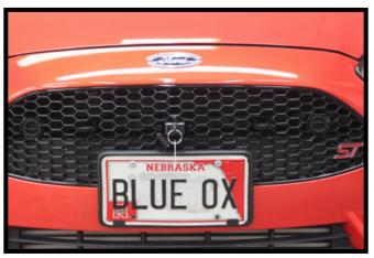
17. Hold the fascia as close to its original position, mark and trim the fascia around the convenience links and attachment tabs. Reinstall the fascia and headlights.
