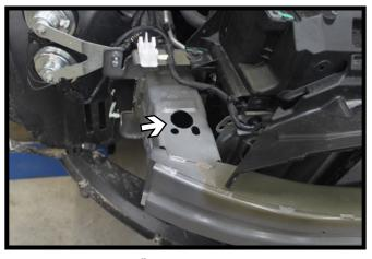
10. Using a 1-1/4" hole saw, drill an access hole on top of the bumper as shown. Do this on both sides of the vehicle.
