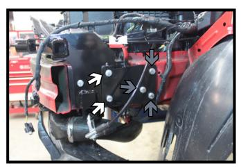
13. Using a 13/32" drill bit, drill the back baseplate holes thru the frame. Bolt the support bracket to the baseplate/frame with 3/8"-16 x 2" bolts, 3/8" lock washers and 3/8" nut plates (white).
