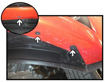
Using a 7MM socket, remove the five (5) screws from the underside of the fascia.
