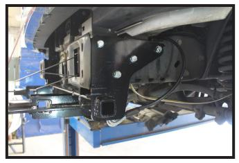
5. Using a 1/2" drill bit, continue drilling the remaining outside holes thru the frame on each frame rail. Install a 1/2"-13 x 1-1/2" bolts with a 1/2" lock washers into the holes and secure with 1/2" nut plates on the inside of the frame. Fully tighten all fasteners.
