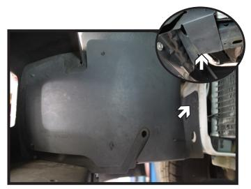
2. Remove the two (2) push pins from the plastic sheilding. Do this on both sides of the vehicle. The sheilding will not be reinstalled.
