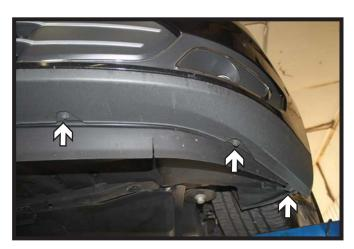
Using a 8MM socket, remove the seven (7) screws from the underside of the fascia. There are three (3) on each side and one (1) in the middle.
