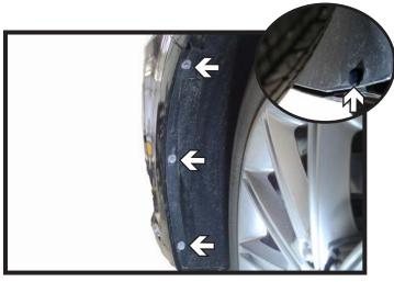
Using a 5.5MM socket, remove the three
