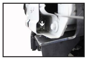
10. On the driver side bumper, using a chisel or flat screwdriver, remove the nut welded on the inside of the bumper for bolt clearance on step #13.
