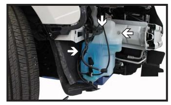
On the passenger side, using a 10MM socket, remove the three (3) screws from the washer reservoir. There are two (2) on the front and one (1) on the backside. Disconnect/plug all lines and set reservoir aside.
