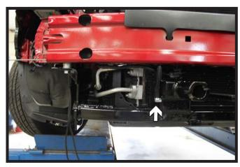
13. Using a 17/32" drill bit, drill a hole thru the bumper using the tube as a guide. Install a 1/2" x 5" bolt with flat and lock washer into the hole and a 1/2" nut plate in the bumper. Depending on the fit, 1/2" flat washers may need to be used in between the bumper and tube. Do this on both sides of the vehicle.
