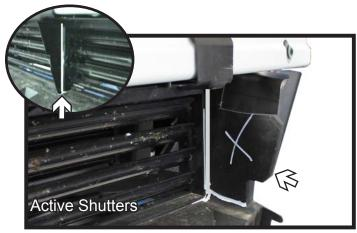
8. **Non-Active Shutters:** Trim the plastic shrouding off just below the bumper as shown for baseplate clearance. Do this on both sides of the vehicle.
