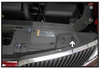
Using a 10MM socket, remove one (1) bolt from the top of the fascia (white).
