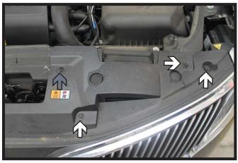
Using a 10MM socket, remove the six (6) screws from the top edge of the fascia.
