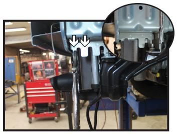
11. Bend the first two (2) tabs of the frame back at a 90° angle for baseplate clearance. Do this on both sides of the vehicle.
