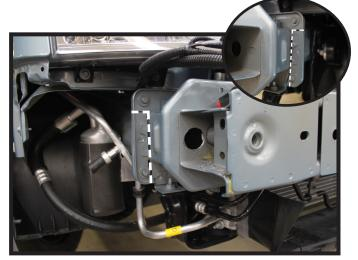
8. Using a reciprocating saw, trim the frame extension on both the driver and passenger sides as shown.
