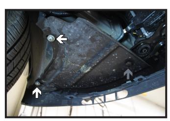
3. On the underside of the fascia on the driver side only, using a T30 Torx, remove the two (2) screws (white). Then remove the push pin (gray).
