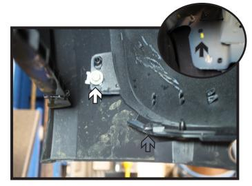
4. Using a 10MM socket, remove the screw from the inside corner of the fascia (white). Then release the clip below (gray). Further up on the inside of the fascia above the screw, release the yellow clip holding on the fender flare (black). Do this on both sides of the vehicle.
