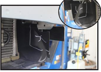
10. Trim the air shrouds on both sides of the vehicle as shown for baseplate clearance.
