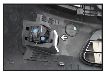
15. On the backside of the fascia, trim the edge of the fog lamp housing as shown. Do this on both sides of the fascia. Reinstall the fascia and plastic covers.
