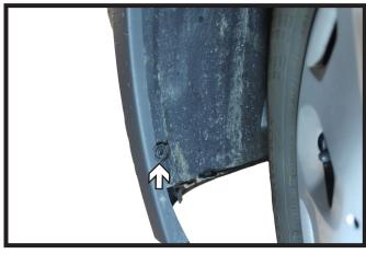
Using a Philips screwdriver, remove the screw from the outer edge of the wheel well. Do this on both sides of the vehicle.
