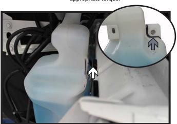
Mark and trim the front tab of the washer fluid reservoir (gray). Reinstall the reservoir, using the supplied 1/4" washers as a spacer on the top rear hole (white).
