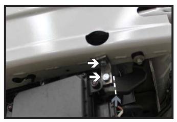
5. **ACC Models:** Align the support bracket as shown, mark holes, then using a 1/4" drill bit, drill the two (2) holes. Install 1/4"-20 x 3/4" bolts and 1/4"-20 nuts (white). Using a reciprocating saw trim off the outer edge (gray).
