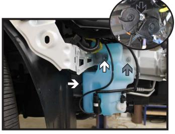
Using a 11MM socket, remove the two (2) screws from the inner edge of the washer fluid reservoir (white). Then using an 8MM socket, remove the outer screw (gray). Disconnect all lines and set reservoir aside.
