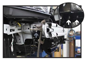
7. Center the baseplate between the frame rib on each side (gray). Level the baseplate and securely clamp in place. On the underside of the baseplate, using a 17/32" drill bit, drill the bottom two (2) holes thru the frame. Install 3/8"-16 x 2-1/2" bolts with 3/8"-16 nut plates into the holes, using the opening in the bumper for nut plate installation (white). Do this on both sides of the vehicle. Tighten all fasteners.
