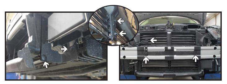
6. **Taurus Models:** Remove the two (2) push pins from the side of the air dam (left). Do this on both sides of the vehicle.
