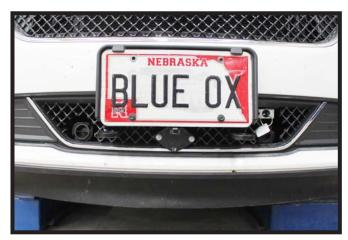
14. Hold the fascia up as close to its original position as possible. Mark and trim around the attachment tabs and convenience links. Reinstall the fascia.
