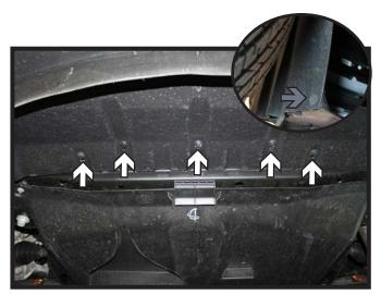
3. Remove the five (5) push pins from the underside of the fascia (white). Then using an 8MM socket, remove screw on the inner edge of the wheel well, there is one (1) on either side of the vehicle (gray). Remove the fascia from the vehicle disconnecting all electrical connections and set aside.
