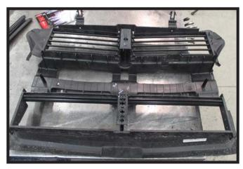
12. **Taurus Models:** Lay the air shutter on a flat, sturdy surface. Insert a flat screwdriver into the lower portion of the air shutter bracket and pop up. (Left)
