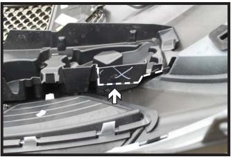
10. On the backside of the fascia, mark and trim the fascia as shown. Do this on both sides of the fascia
