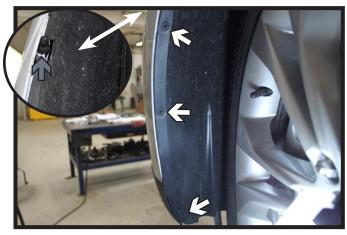
2. In the wheel well, using a 5.5MM socket, remove the three (3) screws from the outer edge (white). Remove the push pin from the upper outer edge (gray). Do this on both sides of the vehicle.
