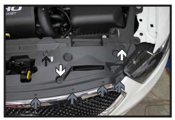
On the top edge of the fascia, using a 10MM Socket, remove the two (2) screws (white). Remove the one (1) push pin (black). Then using a phillips screwdriver, remove the four (4) screws (gray). Do this on both sides of the vehicle.
