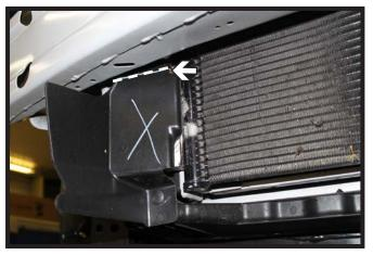
Taurus SHO Models: On the passenger side, using a utility knife, trim off the plastic shrouding from the underside of the bumper.
