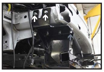
8. Using a 17/32" drill bit, drill the remaining three (3) holes thru the frame and bumper. Install two (2) 3/8"-16 x 1-1/4" bolts and 3/8"-16 nut plates into the top holes (white). In the lower bumper hole, install a 3/8-16 x 2" bolt with 3/8"-16 nut with 3/8" washers in between the bumper & baseplate as a spacer (gray). Do this on both sides of the vehicle. Tighten all fasteners.
