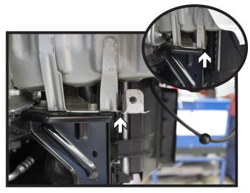
13. On the passenger's side only, use a reciprocating saw to remove the washer reservoir bracket and horn front bracket.
