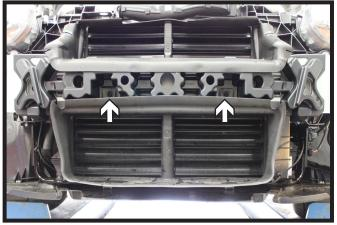
9. Using a T30 Torx, remove the flexible intake cover. The intake cover will not be reinstalled.
