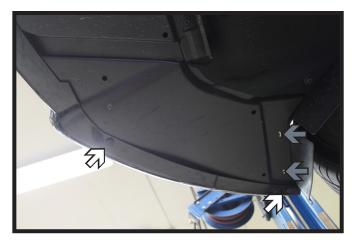
On the underside of the fascia, using a flat screwdriver, remove the two (2) pushpins from the outer edge (white arrows). Using a T27 torx, remove the two (2) rear screws (gray arrows). Repeat this on the other side of the vehicle.
