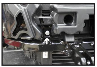
15. On the front of the baseplate, using the attachment tab as a guide, drill out the bumper with a 13/32" drill bit. Insert a 3/8"-16 x 1-1/2" hex bolt and 3/8" lock washer with a 3/8"-16 lock nut. Do this on both sides of the vehicle.
