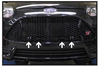
20. Align the fascia as close to its original position and trim the opening for the attachment tabs and convienence links with a utility knife. Reinstall the fascia.
