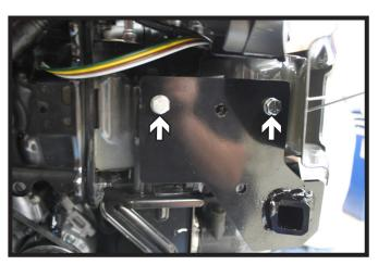
14. Slide the baseplate onto the vehicle until the top back hole is aligned with the top back existing hole on the frame webbing. Insert a 3/8"-16 x 1-1/2" hex bolt and 3/8" lock washer with a 3/8"-16 nut plate. Also secure the top front hole the same way. **DO NOT** tighten bolts all the way, wait until directed to do so. Do this on both sides of the vehicle.
