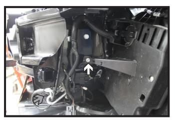
19. Bend the webbing bracket back to its original position and reinstall the 10MM bolt (white).
