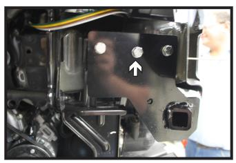
16. Insert a 3/8"-16 x 1-1/2" hex bolt and 3/8" lock washer with a 3/8"-16 nut plate into the middle hole. If necessary drill out any obstructions with a 13/32" drill bit. Do this on both sides of the vehicle. Tighten down all hardware to specified torque.
