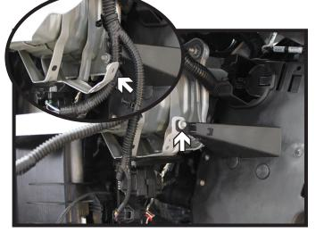
On the driver's side, use a 8MM socket to remove the bolt from the frame webbing. Once the bolt is removed, bend the webbing outward with a pair of large vice grips far enough to fit the baseplate on top of it.
