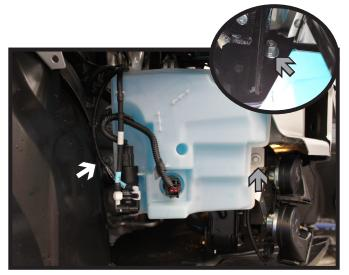
17. Reattach the washer reservoir on the passenger's side. Use the existing bolt in the back (white arrow). Use a 3/8"-16 x 1" hex bolt with a 3/8" flat washer and a 3/8" hex nut and secure the front hole to the baseplate (gray arrow).
