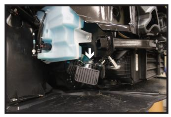
18. To reattach the horn, use the existing hole in the frame webbing on the passenger's side and the existing hole on the horn bracket, and insert a 1/4-20 x 3/4" hex bolt with a 1/4" lock washer and 1/4-20 nut. Reattach all electrical connections.
