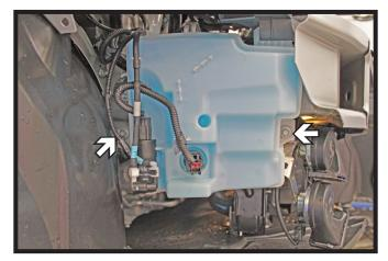
Using a 10MM socket, remove the two (2) bolts from the washer reservoir on the passenger's side. Disconnect all electrical connections. Remove and plug the fluid lines.
