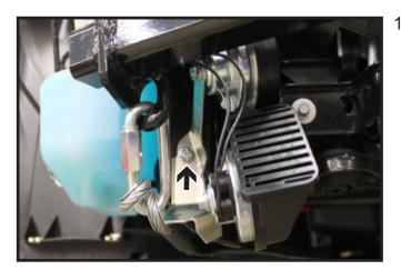
17. On the passenger side, reinstall the horn to the vehicle. Use one of the existing holes on the frame below the baseplate with a 1/4"-20 x 3/4" bolt and 1/4" nylon nut. Bend the bracket if needed to insure that the horn drains if exposed to water.
