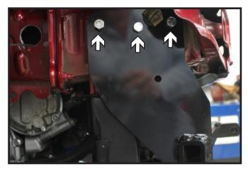
Using the existing holes in the frame, bolt the baseplate to the vehicle with the 3/8"-16 x 1-1/2" bolts and 3/8" nut plates. Ream out the holes if necessay for bolt clearance. Do this on both sides of the vehicle. Make sure baseplate is level before tightening down fasteners.
