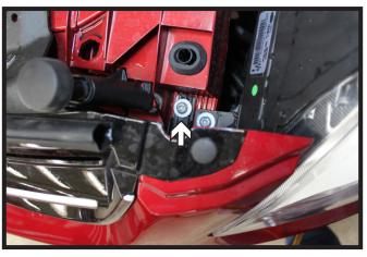
2. Using a T27 Torx, remove the inner screw behind the headlight from the fascia. Do this on both sides of the vehicle.
