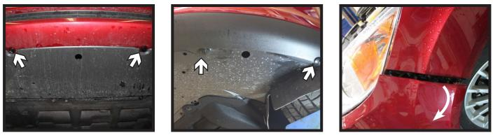
4. On the underside of the fascia, remove the two (2) push pins from the center (left). Then remove the four (4) remaining push pins, two (2) on either side of the center push pins (middle). Pull the corners of the fascia out and forward to unclip and remove from the vehicle (right).
