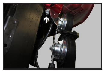
6. Using a 10MM socket, remove the screw from the backside of the horn bracket and set the horn assembly aside.
