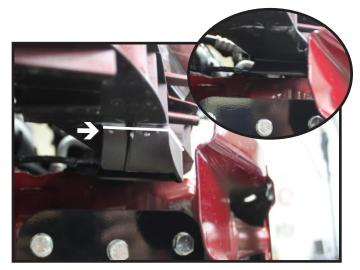
14. On the passenger side, trim the plastic flange above the baseplate for clearance of the washer fluid reservoir.
