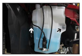
On the passenger side, reinstall the washer fluid reservoir. Reuse one (1) of the existing screws on left side (white). Then a 3/8"-16 x 1" bolt, 3/8" flat washer and 3/8" lock nut on the right side (black).
