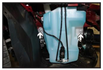
5. On the passenger side, using a 10MM socket, remove the two (2) screws from the washer fluid reservoir. Disconnect lines and set reservoir aside.
