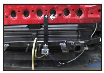
18. Optional: Install the breakaway bracket to the metal bumper with a #10-16 x 1" Self Drilling screw (white). Attach the breakaway to the bracket with a 1/4"-20 x 3/4" bolt and 1/4" lock nut.
