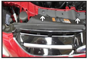
1. Remove the two (2) push pins from the top back edge of the fascia. Do this on both sides of vehicle.
