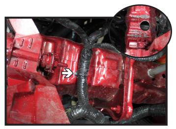
Behind the headlights, unclip the wiring loom to expose the existing hole. Using a 1-1/4" hole saw, drill the existing hole for access to install the baseplate nut plate. Do this on both sides of the vehicle.
