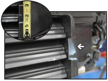
Hold up the baseplate to the vehicle and mark the shutter for cutting. The dimensions should be roughly 1-1/2" from the bottom and 3-1/4" to top of the cut. Trim both ends of the shutter to clear the baseplate.
