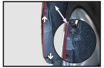
3. Using a T27 Torx, remove the two (2) screws from the outer edge of the wheel well (white). Above the screws where the fascia meets the fender remove the push pin (gray). Do this on both sides of the vehicle.
