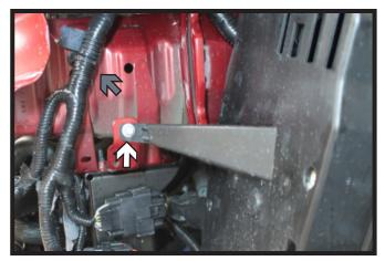
7. On the driver side of vehicle, using an 8MM socket, remove the screw from the air box. Then bend the metal tab away from the vehicle for baseplate clearance (white). Also remove the wire loom from the frame and push aside (gray).
