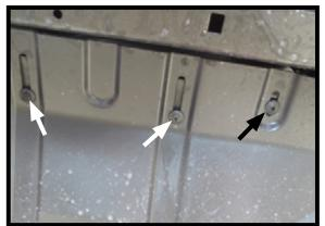
5. On the underside of the vehicle there are five (5) push pins. There is one (1) in the center and two (2) per side. Use a Phillips screwdriver to remove them.
