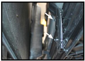
9. On the backside of the air shutter there are three (3) clamps. Tightly squeeze the clamp button to release. There are three (3) buttons on each clamp, two (2) towards the bottom and one (1) towards the top.
