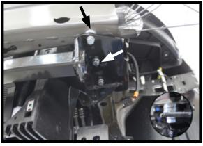
14. Drill the three (3) bottom holes using a 13/32" drill bit.
