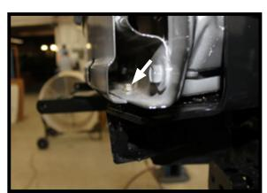
15. On the driver's side only: Use a flat chisel and hammer to remove the nut that is located on the outer edge inside the vehicle frame rail.
