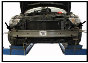
12. Clamp the baseplate securely into place and verify it is properly aligned.
