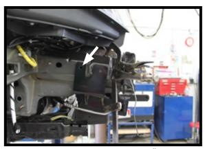
13. Drill one (1) hole using a 13/32" drill bit. Do this on both sides of the vehicle. Recheck the baseplate for proper alignment. After making any adjustments necessary, drill the second hole on each side.
