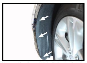
2. Remove the three (3) bolts located on the outer edge of the wheel well area with a 5.5MM socket. Do this on both sides of the vehicle.
