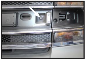
Once the center panel has been removed, use a 10MM socket to remove the bolt. There is one (1) on each side of the vehicle.
