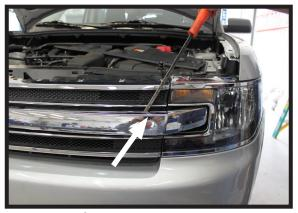
4. Use a flat screwdriver to gently pry the center panel out.
