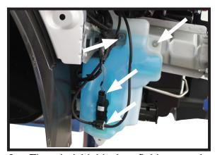
9. The windshield wiper fluid reservoir needs to be removed on the passenger side. Unplug all electrical components and remove the bolt on the top, right side using a 8MM socket. Using a 11MM socket, remove the other two (2) bolts.
