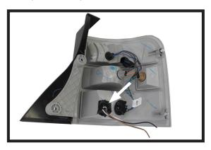
Drill a hole according to the tail light wiring kit.
