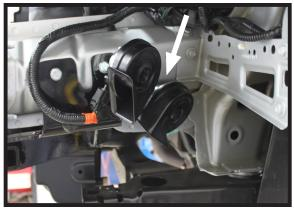
Reinstall the horn to the original location. It may require bending slightly.
