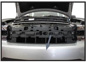
7. The front fascia can now be removed by pulling firmly outward.
