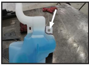
16 . Prior to reinstalling the windshield wiper reservoir, notch as shown above.
