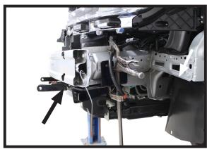
10. Clamp the baseplate securely into place and verify it is aligned evenly.
