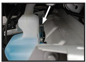
17. Place seven (7) 1/4" flat washers behind the reservoir on the inner most side prior to tightening the existing bolts.
