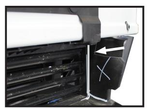
7. On both sides notch the plastic tab from the top of the tab to the bottom as indicated in the image above.
