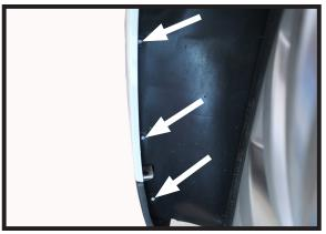
2. Using a 5.5MM socket, remove the three (3) bolts in the wheel well area. Do this on both sides.
