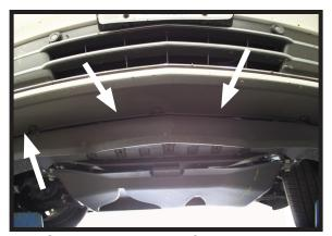
3. On the underside of the vehicle use a 5.5MM socket to remove seven (7) bolts. There are three (3) on per side and one (1) in the center.
