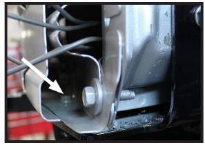
11. On the driver's side only, use a flat chisel to remove the nut that is located on the outer edge inside the vehicle frame rail.
