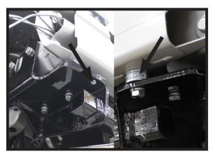
12. Continue using the 13/32" drill bit and drill the bottom, front hole.
