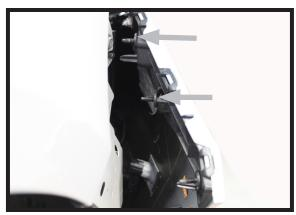
Unclip the fascia on both sides of the vehicle. Using a 10MM socket, reach inside, on the backside of the fascia remove three (3) bolts.
