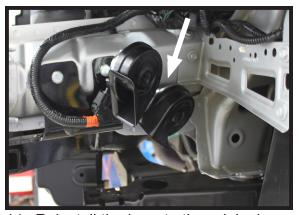
14. Reinstall the horn to the original location. It may require bending slightly.
