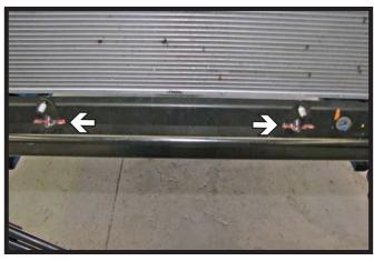
Using a reciprocating saw, cut off the tabs that the lower coolant line were attached to, being careful not to cut into the radiator.
