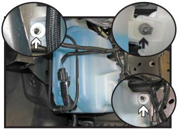
On the passengers side, using an 8MM socket remove the bolt on the top (black). With the 10MM socket remove the two (2) nuts on either side (white). Unplug the hoses and electrical lines and remove the washer fluid reservoir.
