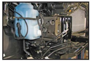
18. Reinstall the washer fluid reservoir, cruise control box. Hold the fascia as close to its original position. Mark and trim for the attachment tabs and conveinence links. Reinstall the fascia
