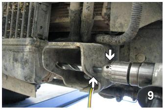
Align the baseplate with the existing holes in the frame, With the baseplate as a template, use a 17/32" drill bit to ream out the holes on both sides of the frame rail if needed. Do this on both sides of the vehicle.
