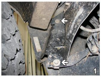
Using a 13MM socket, remove two metric bolts located just forward of the front tire. Do this to both sides of the vehicle. Set bolts aside to be reinstalled later.
