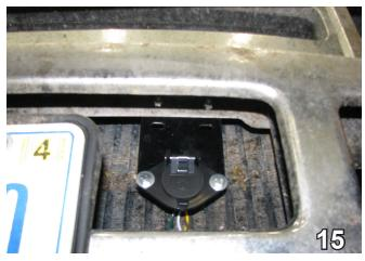
15. Install the electrical plug on the front of the fascia.
