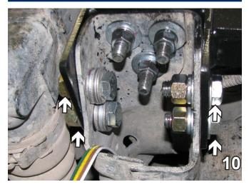
10. Loosely install all four 5/8-11 x 2" bolts with 5/8 flat washers attached to 5/8" lock washers and 5/8-11 hex nuts on the inside. Then use Loctite Red and tighten. Do this on both sides.
