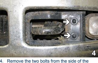
4. Remove the two bolts from the side of the tow hook cover. Do this on both sides of the vehicle. Set the bolts aside to be reinstalled later. Some vehicles may need to have the fog lights removed. If so use an 8MM socket to remove the three metric bolts on both sides.
