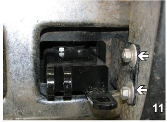
Reinstall the bolts attaching the tow hook covers. Do this on both sides.
