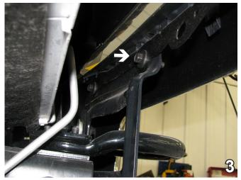
3. Remove the bolt which is exposed after removal of the cover. Set the bolt aside to be reinstalled later.
