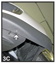
3. **MKS** models: On the underside use an 8MM socket to remove the bolts (white arrows). There is one (1) bolt on the outermost edges of the fascia, figure 3C, one (1) directly in the center, figure 3A, and also one (1) between the push pins, figure 3B.
