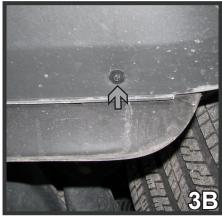
3. **MKT models:** In front underneath, remove three push pins from the center. Using a 5.5MM socket, remove one bolt on each side (gray arrow). Pull fascia corners out to the side of the vehicle to unsnap, then pull forward. Set fascia, pins and bolts aside carefully to be reinstalled later.
