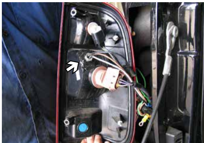
Possible Location for the BX8869 Bulb and Socket Wiring Kit.
