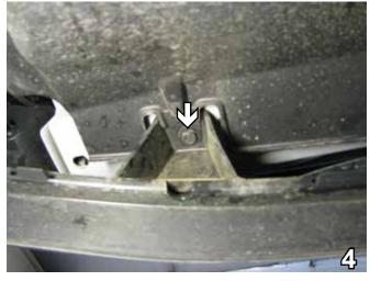
Remove three bolts from across the bottom corner of the fascia, using the 10mm socket. Set bolts aside to be reinstalled later.
