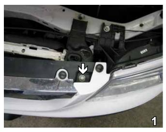
On the upper corner of grille, use the 10mm socket to remove one metric bolt. Do this to both sides of the vehicle. Set bolts aside to be reinstalled later.
