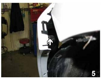
5. Reach in behind the fascia and push the clip holding the fascia down to release. Do this to both sides of the vehicle.
