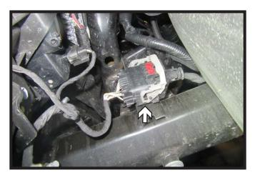
3. Unplug the electrical from the driver side of the vehicle. Remove the bumper/fascia and set aside to be reinstalled later.
