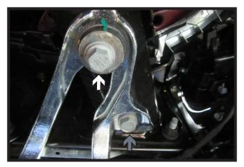
4. **Trucks with Tow Hooks:** Using an 18MM socket remove the front bolt (white) and then using a 21MM socket remove the back bolt (gray) attaching the tow hook to the frame. Do this on both sides of the vehicle. The tow hooks will not be reinstalled.
