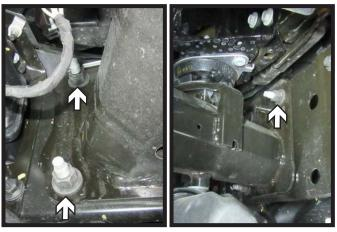
Using an 18MM socket, remove the three (3) bolts from the bumper. Do this on both sides of the vehicle.
