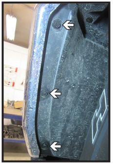
Using an 8MM socket, remove the three (3) bolts from the wheel well. Do this on both sides of the vehicle.
