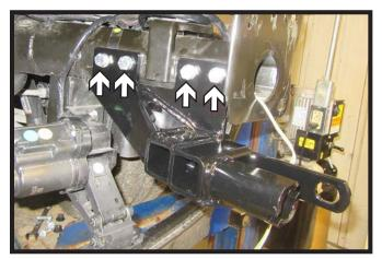
Using a 1/2" drill bit, drill the four (4) holes on the side of the frame starting with the back hole. Install 1/2" bolts with lock washers and whiz nuts. Do this on both sides of the vehicle.
