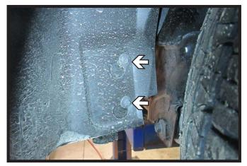
Using an 8MM socket loosen the two (2) bolts holding the wheel well liner and remove to allow for easier drilling. Set aside to be reinstalled later. Do this on both sides of the vehicle.
