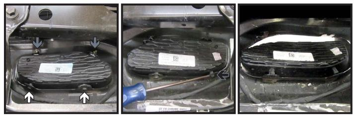
9. Trucks without Tow Hooks: The tow hook covers will need to be removed to allow the baseplate to come through the fascia. Using an 8MM wrench loosen the two (2) bolts (white) on the bottom of the cover. Remove the two (2) clips (gray) from the top side of the cover. Using a flat head screwdriver pull off the rings (black) from the bottom two (2) bolts. Then push the cover towards the front of the fascia and remove. Do this on both sides of the vehicle.
