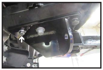
Using a 1/2" drill bit, drill the back hole on the underside of the baseplate. Install one (1) 1/2" bolt with lock washer and whiz nut. Do this on both sides of the vehicle.
