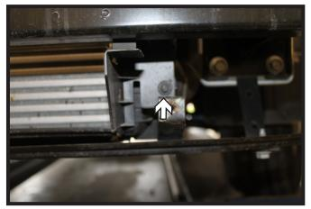
8. Using a 8MM socket, remove the screw from the lower plastic shielding. Do this on both sides of the vehicle.
