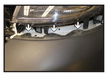
Underneath the headlight, using a 30 Torx or 5/32" allen wrench, remove the three (3) screws. Do this on both sides of the vehicle.
