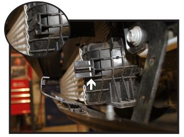
10. Cut the plastic reinforcement tab back flush to the base. Do this on both sides of the vehicle.
