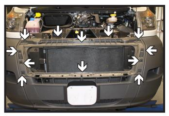
2. Using a T30 Torx, remove the twelve (12) screws from the fascia.
