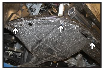
12. On the passenger side, using a 8MM socket, remove the three (3) screws from the plastic shielding. Underneath the shielding, using a 13MM socket, remove the bolt from the fascia reinforcement and set aside.
