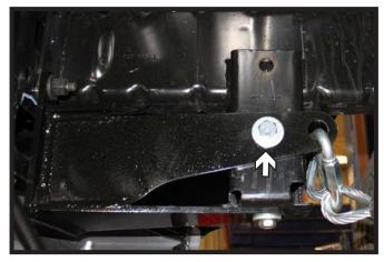
Install the 1/2" hardware into the rear baseplate hole thru the extension. Fully tighten all hardware. Do this on both sides of the vehicle.
