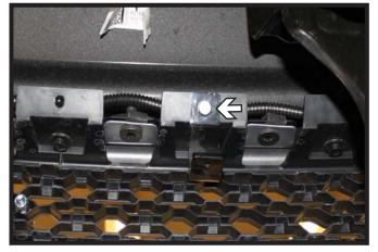
7. **Optional Breakaway:** On the inside of the lower grille remove the push pin at the desired location and install the bracket with the 1/4" hardware provided. Trim the lower grille and install the breakaway to the bracket with the 1/4" hardware provided. 8. Reinstall the lower wheel well liners.
