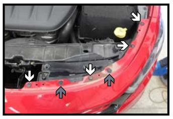
2. On top side of fascia, remove the four (4) push pins (white). Using a 10MM socket, remove the two (2) screws (gray). Do this on both sides of vehicle.
