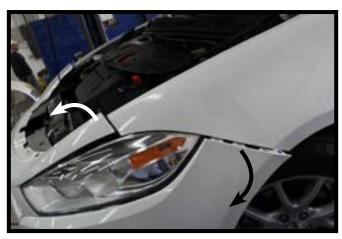
5. Pull edges of fascia up and out to separate from body. Repeat on other side of vehicle. Then remove the fascia from vehicle disconnecting any electrical connections and set aside.
