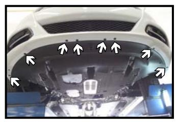
4. Using a 8MM socket remove the eight (8) screws from underneath the fascia.
