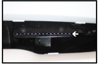
Using a reciprocating saw, trim the tow hook plates flush with the bottom of the bolts. Do this on both sides of the vehicle.
