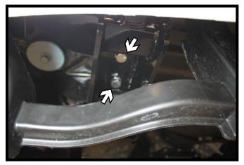
7. Using a 17/32" drill bit, drill the bottom two (2) holes of the baseplate thru the frame. Install 1/2"-13 x 1-1/2" bolts with 1/2" lock washers into the holes with 1/2" nut wires on the inside of the frame and tighten. Remove the clamps. Do this on both sides of the vehicle.
