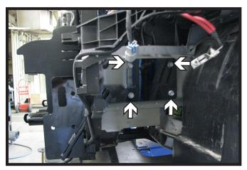
Slide the baseplate onto the vehicle. On the driver side, install four (4) 8MM-1.25 x 35MM bolts into the existing holes.
