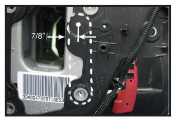
10. Measure from the inside of the frame over 7/8", then using the 1-1/4" holesaw bit trace the diameter. On the lower bumper bolt hole also trace the diameter of the holesaw bit. Connect the outside edges.
