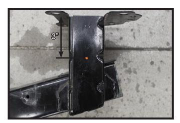
13. On the top side of the bumper, place a mark 3" from the back and centered across. Drill out using a 1-1/4" holesaw. Do this on both sides of the bumper.
