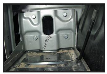
19. On the driver side, remove the four (4) 8MM bolts from the baseplate. Reinstall the battery tray with the 8MM bolts and the 8MM lock washers provided with loctite. Reinstall the battery and terminal connections.
