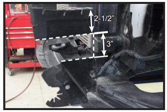
14. On the plastic deflectors, make a notch down 2-1/2" from the top and 3" high from the front to the back for baseplate clearance. Do this on both sides of the vehicle.
