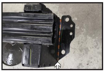
12. Using a reciprocating saw, trim off the outer flanges of the bumper flush with the sides. Do this on both sides of the bumper.
