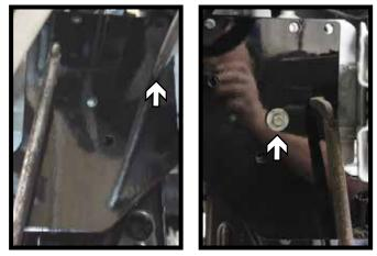
15. Slide the baseplate onto the frame, line the back of the baseplate with the mark. On the driver side pin to the existing hole in the frame (left). On the passenger side install the washer reservoir bolt into the existing hole (right). Level the baseplate and clamp it to the frame.
