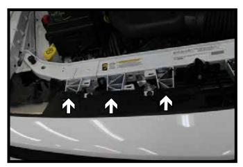
2. Remove the six (6) push pins from the top side of the fascia. Three (3) push pins from both sides of the vehicle.
