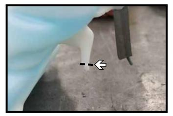
Trim the plastic peg off the washer reservoir. Reinstall the reservoir with the supplied 6MM bolts and spacers. Reattach the power steering pump.
