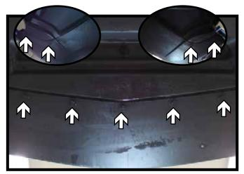
Using a 7MM socket, remove the nine (9) screws from the bottom edge of the fascia. There are two (2) on each side and five (5) in the center.
