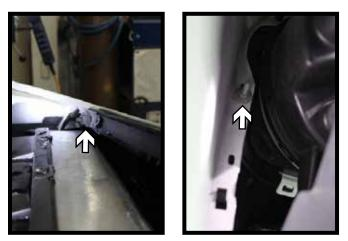
6. Using a 10MM Socket, remove the two (2) nuts from the fascia studs. One (1) is located at on the top side above the headlight (left) and the other in behind the wheel well cover (right). Do this on both sides of the vehicle. Remove the fascia from the vehicle, unhooking any electrical connections from the vehicle.
