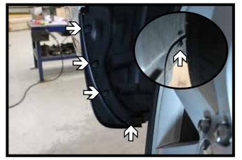
3. Remove the five (5) pushpins from the wheel well. Four (4) from the outer edge and one (1) on the inner bottom edge. Do this on both sides of the vehicle.
