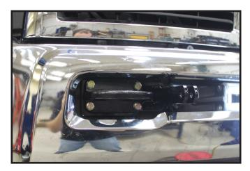
Using a 16MM socket/wrench, install the baseplate and tow hook into the tow hook holes using the 10MM-1.5 x 50MM bolts, 10MM flat washers and existing nuts. Repeat on the other side of the vehicle.
