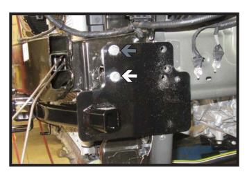
13. Start a 3/8" bolt with lock washer and nut plate in the bottom front hole (white). Using a 3/8" drill bit, drill the top front hole and install the 3/8" bolt with lock washer and nut plate (gray). Remove the 6MM bolt from the existing back hole. Do this on both sides of the vehicle.
