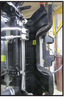
9. Remove the one (1) push pin from the top of the air baffle, lift up on the baffle to remove and set aside to be reinstalled later. Do this on both sides of the vehicle.
