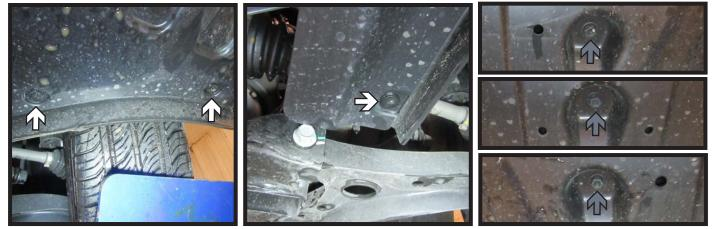
5. Remove the six (6) push pins, three (3) on each side, from the belly pan (white). Then using a 10MM socket remove the three (3) bolts along the center (gray). Remove belly pan and fascia, set aside to be reinstalled later.
