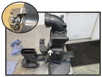
17. Remove the indicated attachment point on the air intake and reinstall on the driver side of the vehicle.
