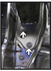
6. Using a 12MM socket, remove the four (4) bolts (white) from the bumper. Using a 10MM socket, remove the one (1) bolt (gray) on the top of the bumper. Do this on both sides of the vehicle. Unclip the wire loom from the bumper. Remove bumper and set aside to be reinstalled later.
