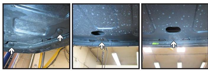
4. Remove the seven (7) push pins from the underside of the fascia. There are three (3) push pins on each side of the vehicle and one (1) in the center.
