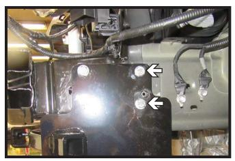
15. Using a 3/8" drill bit, drill the back two (2) indicated holes. Install 3/8" bolts with lock washers and nut plates. Do this on both sides of the vehicle.
