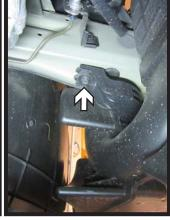
8. Using a 10MM socket, remove the three (3) bolts from the air intake on the driver side of the vehicle. Remove the air intake and set aside to be reinstalled later.
