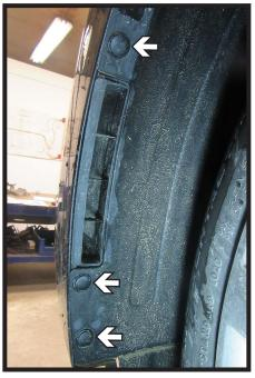
2. Remove the three (3) push pins along the edge of the wheel well. Do this on both sides of the vehicle.
