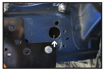
13. On each side of the frame right above the baseplate drill an 1-1/4" hole using a hole saw to use as an the access hole for the nut plates with 14" wire.
