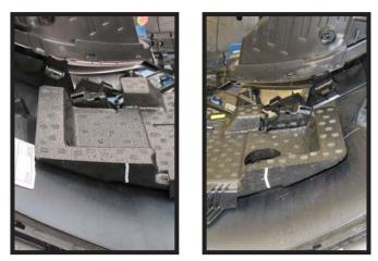
18. Using a reciprocating saw, trim the marked areas on both sides of the fascia.
