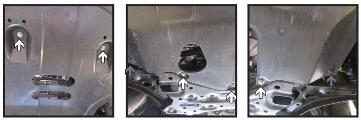
7. Using a 10MM socket, remove the four (4) bolts at the front of the belly pan. There are two (2) on each side of the vehicle (left). Next, remove the two (2) bolts (center white) and the one (1) push pin (center gray) from the back-passenger side of the belly pan. Then, remove the one (1) bolt (right white) and the one (1) push pin (right gray) from the back-driver side of the belly pan. Remove the belly pan and set aside.
