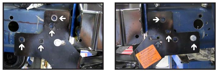
16. Install the baseplate to the frame, aligning the existing holes in the frame to the baseplate. Level and clamp in place. (It is recommended to use the existing bolts to pin the baseplate in place while leveling and clamping, then remove after baseplate bolts are installed)
