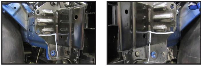
15. Using a reciprocating saw, trim the marked areas on both sides of the bumper horn.
