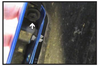
Using a 10MM socket, remove the one (1) bolt from the upper part of the wheel well. Do this for both sides of the vehicle.
