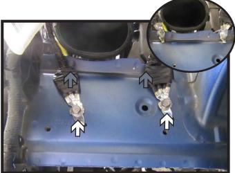
Using a 10MM socket, remove the two
