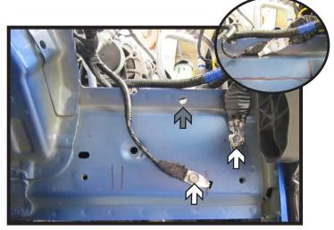
Using a 10MM socket, remove the two
