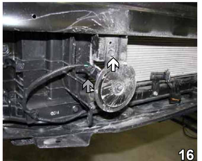
16. Using the 10MM socket, remove the bolt attaching the horn to the bracket (white arrow). Unplug the horn (gray arrow).
