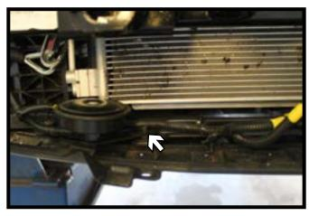
12. **Turbo Models:** Mark the bumper center brace and drill a 1/2" hole thru it to go around the electical rod. Reinstall the brace to the bumper (left). Reinstall the horn to the existing bolt location on the left side of the intercooler (right).
