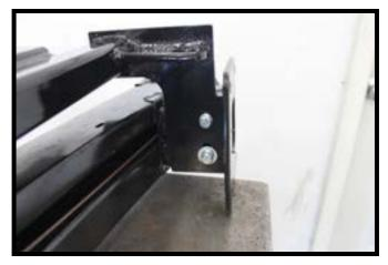
With the bumper upside down, install the baseplate onto the bumper using the 3/8" hardware. Do this on both sides of the bumper. Fully tighten all hardware.
