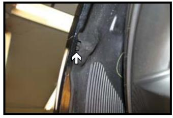
Using a 10MM socket, remove the screw in the wheel well at the fascia/fender joint. Do this on both sides of the vehicle.
