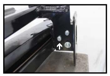
8. Using a 3/8" drill bit, drill the front hole in the baseplate thru the bumper and install the 3/8" hardware. Do this on both sides of the bumper. Fully tighten all hardware.
