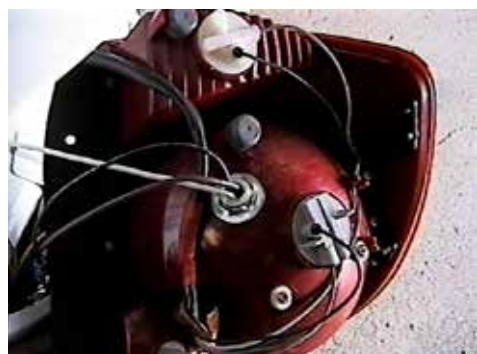
Location of the BX8869 on the driver's side tail light assembly.
