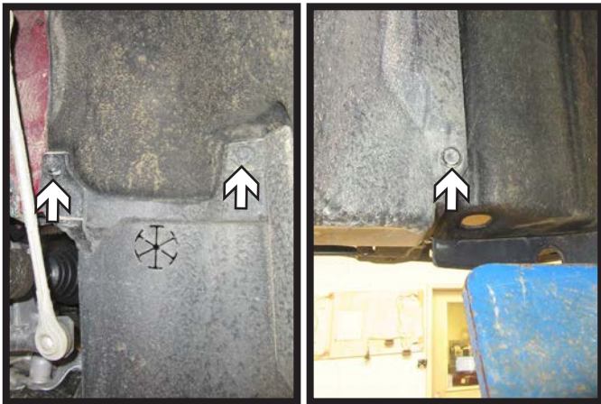
11. Remove the three (3) push pins from the wheel well liner. Do this on both sides of the vehicle. This will allow the belly pan to hang down and give access to the frame.
