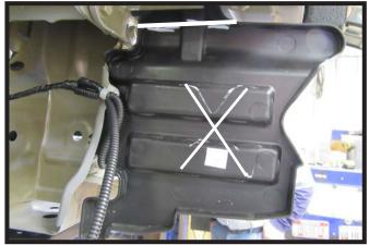
5. Trim plastic piece as indicated so that it is flush with the bumper. Do this on both sides of the vehicle.
