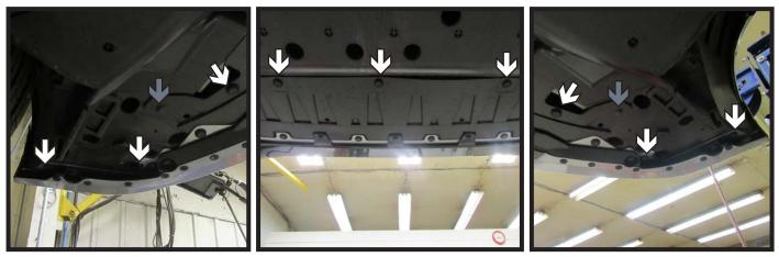
4. Remove the nine (9) push pins (white) from the underside of the vehicle. Then using a Phillips screw driver, remove the two (2) screw (gray). Remove fascia and set aside to be reinstalled later.
