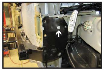
Using a 3/8" drill bit, drill out the center hole. Install the one (1) 3/8" bolt and hardware. Tighten but do not use Loctite<sup>®</sup> Red at this time. Do this on both sides of the vehicle.
