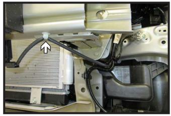
7. Unclip the temperature sensor wire loom from the bumper and unplug sensor.
