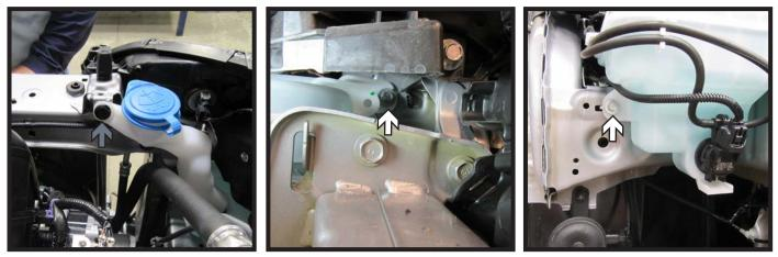
6. On the passenger side of the vehicle remove the windshield washer reservoir. Remove the one (1) push pin (gray) at the top (gray). Then using a 10MM socket remove the two (2) bolts (white) holding the reservoir. Unplug all lines, remove the reservoir and set aside to be reinstalled later.
