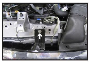
2. Using a 10MM socket to remove the one (1) bolt.
