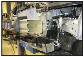
17. Reclip the temperature sensor wire loom to the baseplate. Then using a zip tie attach the sensor to the top of the baseplate.
