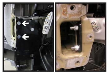
Install the two (2) 3/8" bolts with backing plate and nylon lock nuts on the inside. Tighten fully. Do this on both sides of the vehicle.
