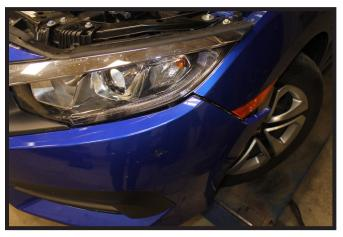
Pull the corners of the fascia away from the vehicle disconnecting any electrical connections and set the fascia aside.
