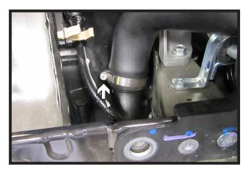
12. Using a 10MM socket remove the bolt attaching the clamp to the coolant tube.
