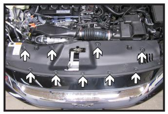
1. Remove the nine (9) push pins from the fascia cover. There are five (5) on driver side and four (4) on the passenger side. Set the cover aside.
