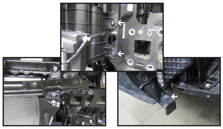
9. Remove the plastic shielding from the vehicle by removing the four (4) push pins. There is one (1) on top, two (2) along the side and one (1) at the bottom. Do this on both sides of the vehicle. The shielding will not be reinstalled.
