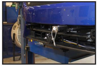
21. **Optional Breakaway:** In the desired location, drill a 1/4" hole thru the fascia lip. Install the breakaway to the fascia with the 1/4" hardware provided.
