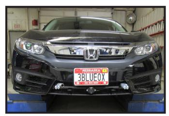
20. Hold the fascia as close to its original position, mark and trim the fascia around the convenience links and attachment tabs. Reinstall the headlights, fascia and fascia cover.
