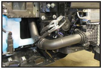
17. Reinstall Coolant tube to the passenger side of the vehicle.
