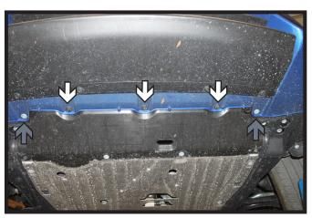
4. Using a 10MM socket, remove the screw (gray) from the underside of the fascia. Then remove the two (2) push pins (left photo). Do this on both sides of the vehicle. Using a T30 Torx, remove the two (2) screws towards the center (gray). Then remove the three (3) push pins (right photo).
