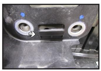
Using a reciprocating saw, trim the hook at the lower bumper bolt location flush with the frame. Do this on both sides of the vehicle.
