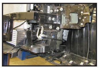
18. Attach the permanent baseplate safety cables to the provided convenience link on the baseplate. The photo above shows the recommended installation of the cables to frame of vehicle. Additional options may interfere with suggested mounting; in this case, secure the cables to a solid piece of the frame as described in the General Information sheet. Be sure the safety cables do not rub against any hoses or moving parts. Do this on **BOTH** sides of the vehicle.
