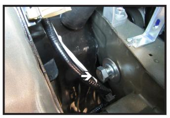
15. Start the 5/8" bolt with flat washer and lock washer. Do not tighten fully. Do this on both sides of the baseplate
