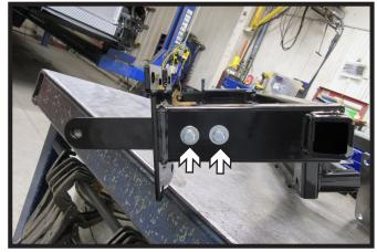
13. Place the baseplate on a flat surface and attach the support strap to the baseplate using two (2) 3/8" bolts. Make sure that the support strap is a straight as possible. Do not tighten fully. Do this for both sides of the baseplate.
