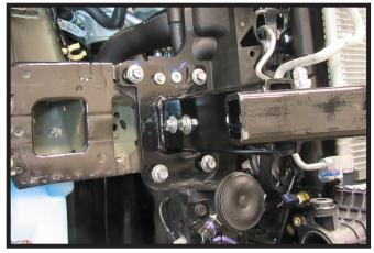
16. Start to remove each bolt that attaches the baseplate to the frame individually and apply Loctite Red and reinstall bolt and tighten to the appropriate torque. Use the following order to remove the bolts individually:10MM, 6MM, 5/8", then finally the 3/8" bolts attaching the support strap.
