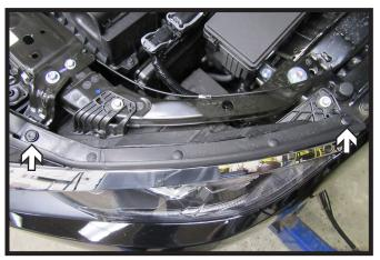
Remove the two (2) push pins from the corner of the chrome strip and unsnap from the vehicle. Do this on both sides of the vehicle.
