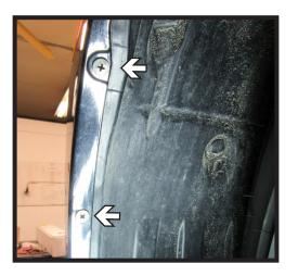
Using a phillips screwdriver, remove the two (2) screws from the underside of the wheel well. Do this on both sides of the vehicle.
