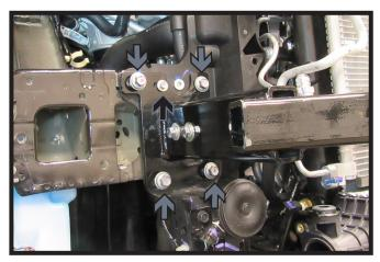
14. Slide the baseplate into position on the vehicle and start the existing 10MM (gray arrows) and 6MM (black arrow) hardware. Do not tighten fully. Do this on both sides of the vehicle.
