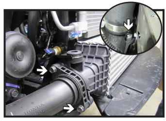
11. Using a 10MM socket remove the three (3) bolts attaching the coolant tube to the passenger side of the vehicle, two (2) in the front and one (1) in the back.
