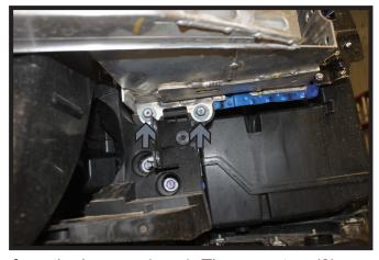
8. Using a 14MM socket, remove the four (4) bolts from the bumper (gray). There are two (2) each on the top side and underside. Using a 12MM socket, remove the bolt from the side of the bumper (white). Using a 10MM socket, remove the bolt from the top side of the bumper (black). Do this on both sides of the vehicle. Set the bumper aside it will not be reinstalled.
