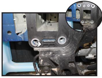
Using a reciprocating saw, trim the hook at the lower bumper bolt location flush with the frame. Do this on both sides of the vehicle.
