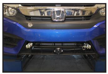
14. Hold the fascia as close to its original position, mark and trim the fascia around the convenience links and attachment tabs. Reinstall the headlights, fascia and fascia cover.
