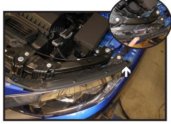
Remove the push pin from the corner of the chrome strip and unsnap from the vehicle. Do this on both sides of the vehicle.
