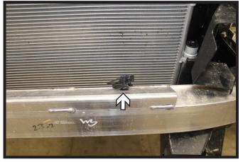
6. Remove the temperature sensor from the bumper and set aside.
