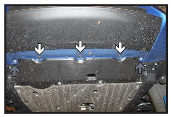
4. Using a 10MM socket, remove the screw (gray) from the underside of the fascia. Then remove the two (2) push pins (left photo). Do this on both sides of the vehicle.
