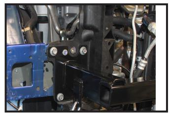
11. Install the baseplate to the vehicle using the existing hardware. Fully tighten all fasteners.
