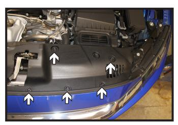
1. Remove the ten (10) push pins from the fascia cover. There are five (5) on each side. Set the cover aside.
