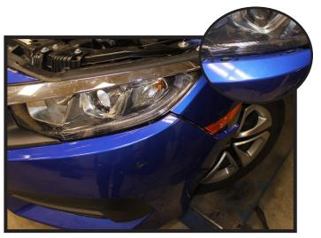
5. Pull the corners of the fascia away from the vehicle disconnecting any electrical connections and set the fascia aside.
