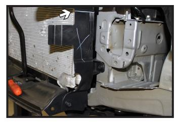
13. Trim the plastic shielding just above the frame pocket, then remove the lower push pins holding it in place. Do this on both sides of the vehicle.
