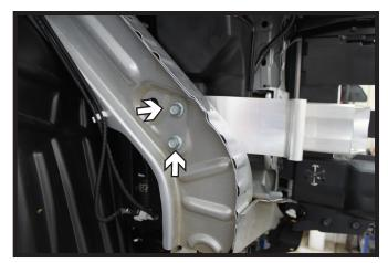
Using a 14MM socket, remove the two (2) bolts from the frame braces. Do this on both sides of the vehicle. The braces will not be reinstalled.
