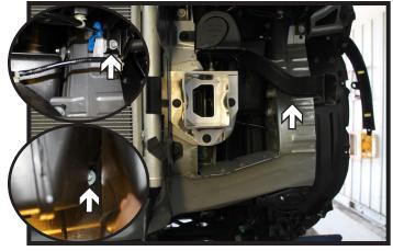
8. On the driver side, using a 10MM socket, remove the two (2) screws from the air baffle and set aside.
