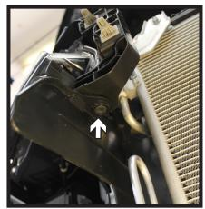
9. Using a 10MM socket, remove the five (5) screws from passenger side headlight assembly. There are two (2) on top, two (2) on the lower face and one (1) on the underside (left & middle). Next to the radiator remove the push pin as shown (right).
