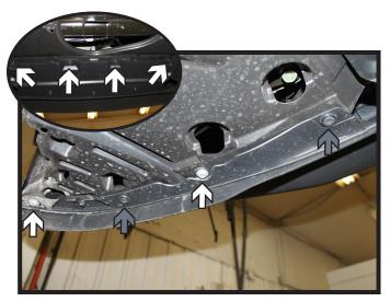
5. Using a 10MM socket, remove the eight (8) screws from the underside of the fascia. There are two (2) in each corner and four (4) in the middle (white).
