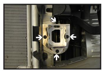
Using a 12MM socket, remove the three
