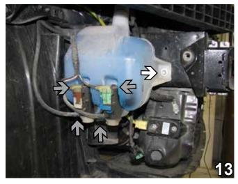
On the passenger side, unhook and plug the hoses and disconnect the electrical wires (gray arrows). Remove one bolt from the side of the metal bumper using the 10mm socket (white arrow). Set bolt aside to be reinstalled later.
