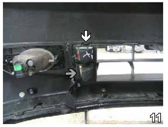
On the driver's side, mark the upper air vent flush with the back side of the grille opening. Using the utility knife, trim the marked area. Some models may need to have the lower air vent removed also (see gray arrow).
