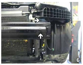
6. Using the 12mm socket, remove two bolts from the metal bumper. Do this to both sides of the vehicle. Pull metal bumper forward to remove. Set bolts and metal bumper aside to be reinstalled later.
