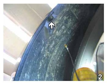
2. Just inside wheel well, on edge of fascia, remove one Phillips screw. Do this to both sides of the vehicle. Set screws aside to be reinstalled later.
