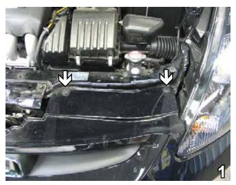
1. On top of the fascia, remove two pushpins between headlights and hood latch. Do this to both sides of the vehicle. Set pushpins aside to be reinstalled later.
