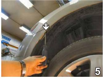
Just forward of the front tire, in an opening between the front fascia and the wheel well, use a Phillips screwdriver to remove the screw. Do this to both sides of the vehicle. Set screws aside to be reinstalled later.
