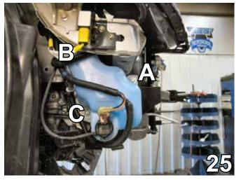
25. Place the windshield washer back to its original position on the passenger's side. Insert the 6MM-1.0 x 30MM hex bolt and fasten with the ½" flat washer and ½" lock washer (A in photo above). Insert and tighten original metric bolt removed earlier (hidden behind hoses in photo above - B). Insert 6MM-1.0 x 45MM hex bolt and fasten with the ½" flat washer and ½" lock washer using the 3/8" pipe spacer between the washer reservoir and the existing location on the frame. (C in photo above).
