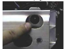
6. Through holes on front side of metal bumper, remove four metric bolts with the 12MM socket and set metal bumper aside.
