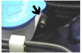
8. Using the 10MM socket remove three metric bolts from windshield washer reservoir, unplug electrical connections and set reservoir on top of engine.
