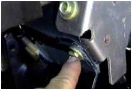
**10.** Using the 12MM socket, remove the four metric bolts from frame end cap, pull forward and set aside, both sides.
