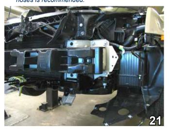
21. Reinstall metal bumper and plastic cover. Tighten all bolts completely. Note: Due to the trimming of the bumper brackets, there will be one less 10mm bolt installed on the bottom of each bumper bracket.
