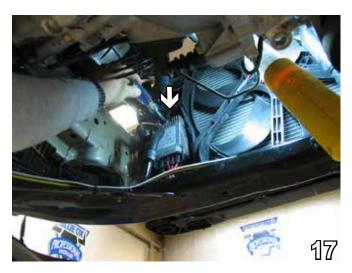
17. Using the 25 Torx socket, remove the bolt in the cut away area above the fan modulator, behind the radiator on the driver's side. Move the fan modulator out of the way to clear the area for baseplate drilling. Set bolt aside to be reinstalled later.
