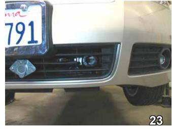
23. Hold the fascia up to its original location, mark and trim the grille with the utility knife as necessary for the attachment tabs to come through. The convenience links will come through the second opening from the top of grille and the electrical rods through the third opening from the top. Reinstall the fascia.
