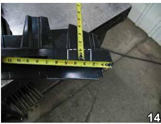
14. On the bottom side of the bumper plastic, measure and mark a rectangle 2 1/2" wide on the raised molding 2 1/4" from the outside edge of the plastic and 1 1/4" high. Trim away the area with the utility knife to open for baseplate installation. Do this to both sides of the plastic. Driver's side is shown in the photo
