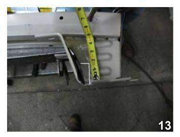
13. Using the reciprocating saw, cut from the outside edge of the bumper bracket's vertical cut, toward the front of the bumper 2" and then across to the inside edge of bumper bracket. Cut along the bumper bracket support contour to the bumper bracket. Finally, complete cutting the rectangular area shown in step 12. Do this to both sides of the metal bumper. Driver's side is shown in the photo.
