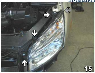
15. Using the 10mm socket, remove three metric bolts from the headlight assembly (see white arrows). Remove one pushpin from the headlight assembly's upper, outside edge (see grey arrow). Do this to both sides of the vehicle. Set bolts and pushpins aside to be reinstalled later.
