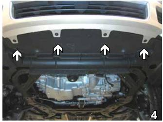
Using the 7mm socket, remove four metric bolts from underneath the center of the fascia. Set bolts aside to be reinstalled later.
