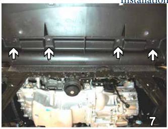
7. Remove four pushpins from the bottom of the bellypan. Pull belly pan down to remove. Set pushpins and belly pan aside to be reinstalled later.
