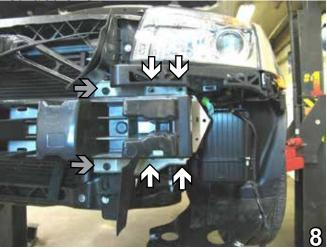
8. Using the 13mm socket, remove four metric bolts from the bumper bracket, two on the top and two on the bottom (see white arrows). Using the 10mm socket, remove two metric bolts from the side of the bumper bracket (see grey arrows). Do this to both sides of the vehicle. Pull the metal bumper forward to remove. Set bolts and metal bumper aside to be reinstalled later.
