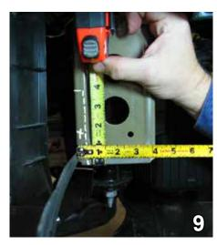
9. Mark the rectangular area on the frame rail end cap, 1/2" from the inside edge and up 4" from the bottom of the frame rail. Trim away the area using the reciprocating saw. This will clear the area for baseplate installation.
