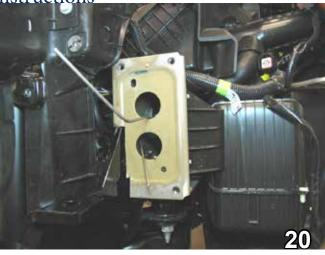
20. Remove the metal bumper. Insert the 3/8-16 nut plates into the frame rail to align with the 3/8-16 x 1 1/2" bolts and tighten with the 9/16" socket. Do this to both sides of the vehicle. Remove the vise grips.
