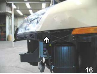
16. Using the 10mm socket, remove one metric bolt from the fender, just forward of the turn signal marker. Disconnect electrical and pull headlight forward to remove. Do this to both sides of the vehicle. Set bolts and headlight assemblies aside to be reinstalled later.
