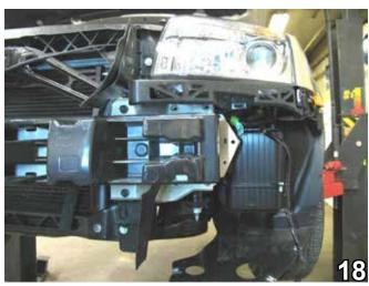
18. Reinstall the metal bumper. Install only two bolts on each side to hold the bumper in place because it will be removed again. It is not necessary to insert the plastic to the front of the bumper at this time.
