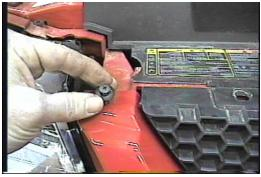
1. Remove the six phillips head push pins from the top side of the grill.
