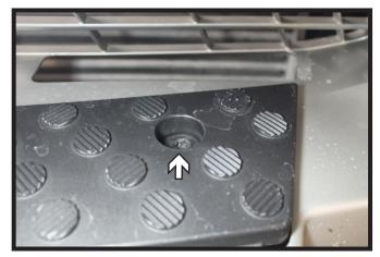
Using a T45 Torx, remove the two (2) screws from the step area on top of the fascia. There is one (1) on each side.
