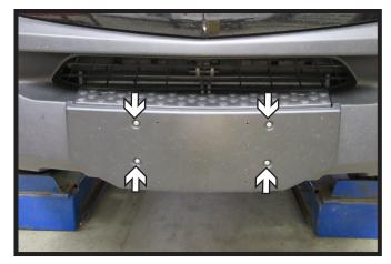
4. Using a T20 Torx, remove the four (4) screws from the front cover.
