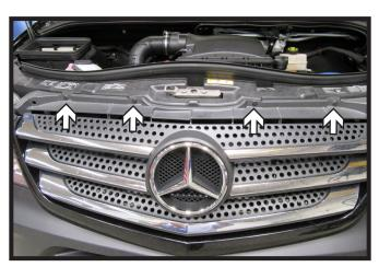
1. Remove the four (4) push pins from the top of the grille.
