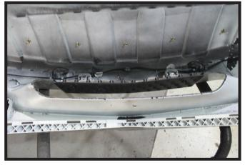
14. On the back side of the fascia, trim off the inner grille at the joint all the way around.
