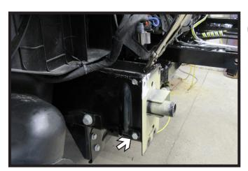
10. Clamp the baseplate to the frame of the vehicle. Using a 3/8" drill bit, drill the lower front baseplate hole thru the frame. Install the 3/8" hardware into the hole and fully tighten. Do this on both sides of the vehicle.
