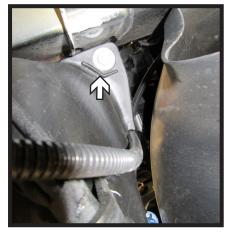
8. On the passenger side, using a 18MM socket, remove the front bolt (middle) from the tank. Then using a 13MM socket, remove the rear bolt (right) and let the tank hang down.
