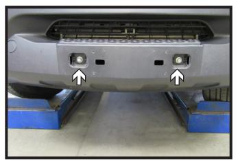
5. Using a 13MM socket, remove the two (2) screws from the front of the fascia.
