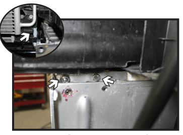
11. Using a 3/8" drill bit, drill thru the frame lips into the top baseplate holes. Install the 3/8" hardware into the top holes and fully tighten. Do this on both sides of the vehicle. Note: the plastic shielding behind may need to be trimmed for easier nut access (inset).
