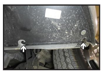
3. Remove the four (4) push pins from the underside of the fascia. There are two (2) on each side.
