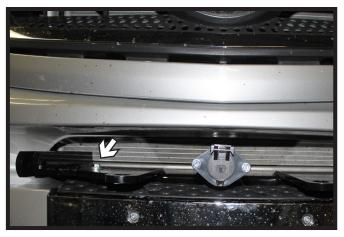
15. Reinstall the bumper. Reinstall the fascia with the 3/4" spacers in the step area bolt recess areas (left). After the fascia is on the vehicle, install the 8MM hardware thru the baseplate into the step area bolt areas and fully tighten.
