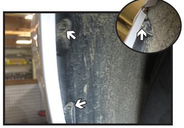
Remove the three (3) push pins in the wheel well. Do this on both sides of the vehicle.
