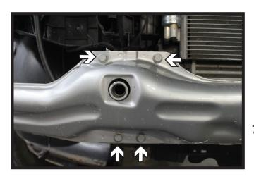
7. Using a 13MM socket, remove the eight (8) bolts from the bumper. There are four (4) on each side.
