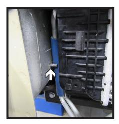
9. On the passenger side, using a 8MM socket, remove the bolt from the compressor line bracket (left). Pull the lines forward, then using a 10MM wrench, remove the nut from the bracket (middle). Set the bracket aside it will not be reinstalled.
