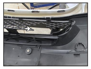
17. Hold front facia up to frame and mark to cut out for clearance around baseplate. After cutting suffient amount for clearance, reattach facia to vehicle.
