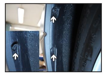
In the front wheel well using a straight screwdriver, turn the two (2) upper and one (1) lower facia pins 90 degrees to unlock and remove. Both driver and passenger sides.
