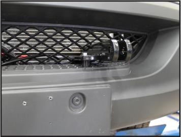
Use 3/4" spacertube before installing 8MM-1.25 x 50MM bolt and 8MM lockwasher, typical both sides.
