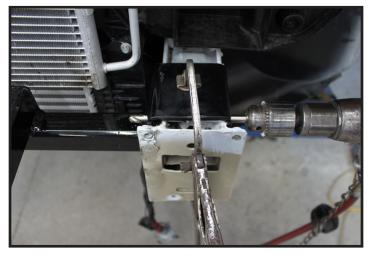
Drill the top front hole thru frame using a 13/32" drill bit. DO NOT drill remaining holes at this time.
