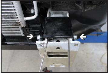
14. On inner frame hole (left) use a 3/8"x1-1/2" bolt, 3/8" lock washer and 3/8"-16 whiz nut. On outer frame (right) use a 3/8"x1-1/4" bolt, 3/8" lock washer and 3/8"-16 whiznut. Repeat on passenger side.
