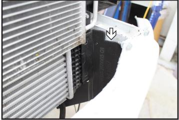
10. Remove cardboard insert from behind bumper on both driver and passenger sides of vehicle.
