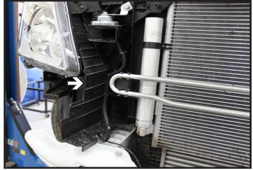
8. Unsnap plastic shrouding on both passenger and driver side.
