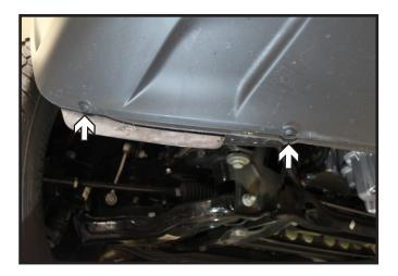
2. At the front of vehicle on the underside of facia using a straight screwdriver, turn the two (2) facia pins 90 degrees to unlock and remove. Both driver and passenger sides.
