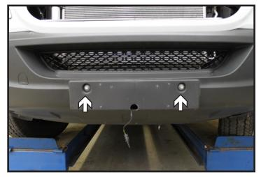
7. Remove the two (2) bolts using a 13mm socket, then remove front facia.
