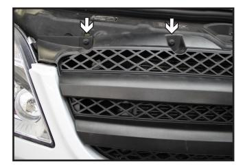
3. On top of the grill locate and remove the two (2) screws using a 25 Torx. Do this on both sides of vehicle. After the four (4) screws are removed the grill can be removed from the vehicle.
