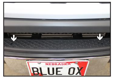
5. Remove the two (2) screws above the license plate bracket using a 25 Torx.
