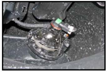
6. Disconnect the fog light and any other electrical connections. Pull the corners of the fascia away from the vehicle and set the fascia aside.
