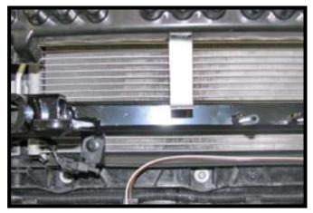
16. Optional Breakaway: Position the bracket in the desired location and drill a 1/4" hole thru the bumper and secure the bracket with the 1/4" x 2-1/4" bolt and lock nut. Attach the breakaway to the bracket with the 1/4" x 3/4" bolt and lock nut.
