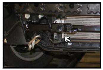
Reinstall the temperature sensor to the bracket on the baseplate.
