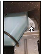
10. On the passenger side, using a 10MM socket, remove the two (2) screws from washer reservoir. Disconnect/plug all connections and set aside.
