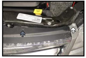
Using a 10MM socket, remove the screw from the top edge of the fascia (white). Then remove the push pin just to the inside of the screw (gray). Do this on both sides of the vehicle.
