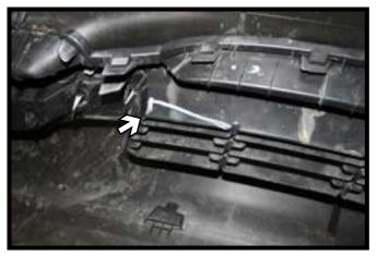
On the backside of the fascia, trim the corner as shown for baseplate clearance. Do this on both sides of the fascia.
