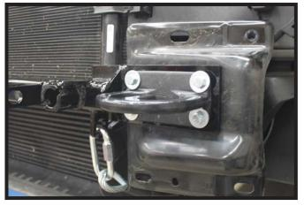
6. Install the baseplate and tow hooks into the tow hook holes with 7/16"-14 x 2" bolts with 7/16" lock washers and lock nuts.
