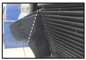
5. **2013 Models:** Trim the lower radiator shroud as shown for D-Link clearance on the baseplate. Do this on both sides of the vehicle.
