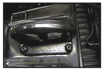
Remove the four (4) bolts from the tow hook, using a 50 Torx and/or a 18MM socket. Do this on both sides of the vehicle.
