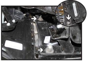
3. Using a 18MM socket, remove the nuts from the backside of the bumper. Do this on both sides of the vehicle. Remove the bumper and set aside.
