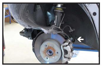
Using a 10MM socket, remove the bolt on the bottom. Do this on both sides of the vehicle.
