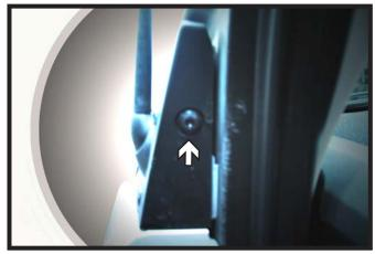
5. Open the door, inside next to the antenna, remove the bolt with a 30 Torx. Do this on both sides of the vehicle.
