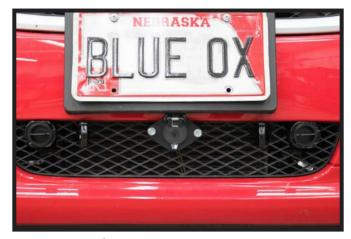
34. Hold the fascia as close to its original position, mark and trim the fascia around the convenience links and attachment tabs. Reinstall the bumper, wheel well covers, tires, fascia, antenna, hood, plastic covers below the doors.
