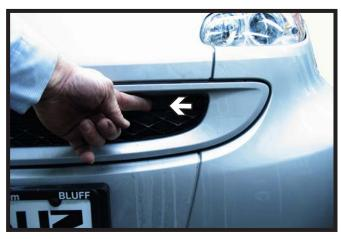
1. Pull the lever in the front to the outside. Do this on both sides of the vehicle. Lift the hood off and set aside.
