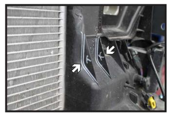
27. On the driver side of the vehicle, use a utility knife to remove the two (2) gussets.
