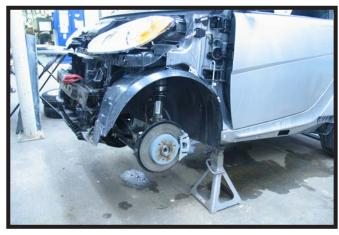
13. Put the vehicle up on jack stands, use a 15MM socket to remove the tire lug nuts. Take the tire off. Do this on both sides of the vehicle.
