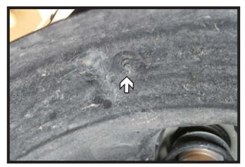
15. Remove push pin from the top of the wheel well. Do this on both sides of the vehicle.
