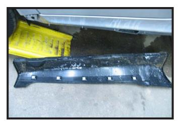
10. Using a flat screwdriver, pry the black covering piece off of each of the five (5) tabs below the door panel. Do this on both sides of the vehicle.
