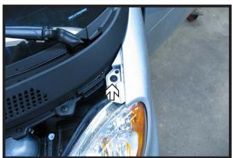
4. Using the 25 Torx, remove the bolt above the headlight. Do this to both sides of the vehicle.
