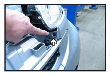
3. Remove the push pin just below the head light. Do this on both sides of the vehicle.
