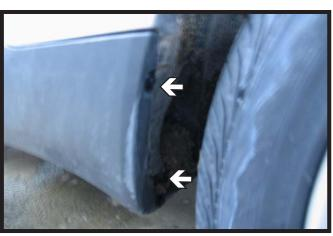
In front of the back tire, remove two (2) push pins. Do this on both sides of the vehicle.
