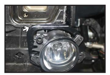
30. 2014 & up Models w/Fog Lights Only: Trim the top of the fog light bezels on both sides of the vehicle as shown for baseplate clearance.
