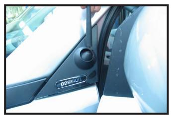
Unscrew the antenna in order to be able to remove the fascia. Also, remove the outer cover by gently pulling on it.
