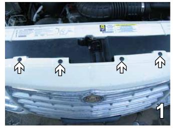
1. Remove the four push pins on the top side of the fascia. Set aside to be reinstalled later.
