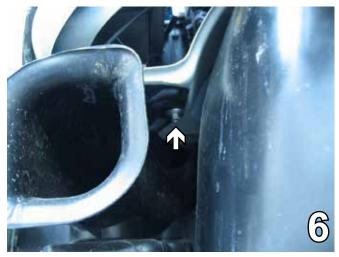
6. On the passenger side, use a 10MM socket to remove the bolt holding the air baffle. Set both the air baffle and the bolt aside to be reinstalled later.
