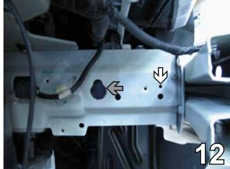
12. On the passenger side, using the 13/32" drill bit, drill another hole in alignment with the washer reservoir existing hole. Also enlarge the existing hole to the back with a 1 1/4" hole saw (gray arrow).
