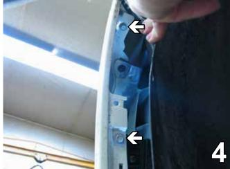
4. Pull the plastic back from the wheel well. Remove two metric bolts with the 10MM socket. Do this on both sides and set aside to be reinstalled later. Pull fascia corners out to the side of the vehicle, then pull fascia forward, unplug electrical connection on passenger's side and carefully set the fascia aside to be reinstalled later.
