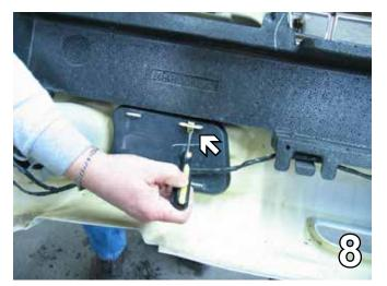
8. With the fascia upside down, push the clip down with the flat screwdriver to remove the black flat pieces. Do this on both sides of the fascia.
