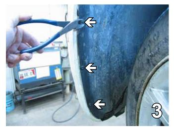
3. Just forward of the front tires in the wheel well, cut the three plastic push poppers with the diagonal cutters. Do this on both sides.
