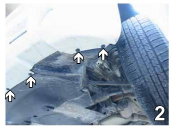
Remove the nine metric bolts from the lower edge of fascia all the way around with the 7MM socket. Set aside to be reinstalled later.
