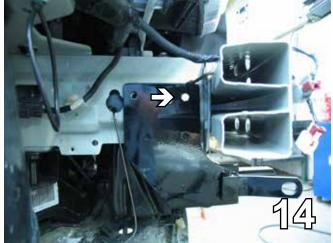
14. On the passenger side, slide the baseplate up from underneath, aline with the drilled hole and the existing washer reservoir hole. Make sure the baseplate is straight and clamp. Using the baseplate as a template, drill the remaining two holes with the 13/32" drill bit.
