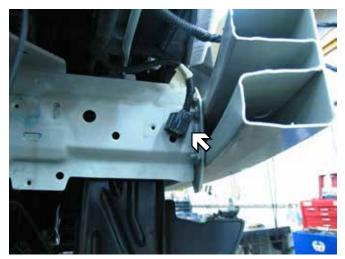
5. On the passenger behind the bumper, disconnect fascia cable from the frame. To prepare area for baseplate install.
