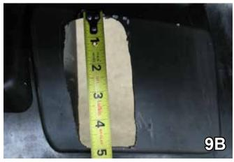
9. Using a hack saw knife, mark and trim out opening in the fascia for the attachment tabs, using the photos above as a template. Do this to both sides of the vehicle. Models that have tow hooks will not need to cut out opening in fascia.
