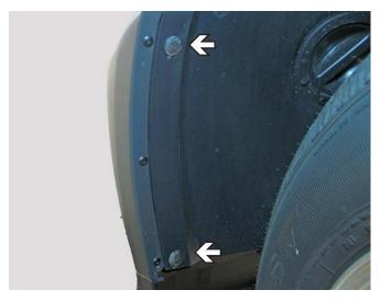
1. **DODGE ONLY:** Using a flat screwdriver, remove two pushpins just forward the front tire, on the wheel well. Set pushpins aside to be reinstalled later. Do this to both sides of the vehicle.
