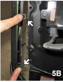
5. **JEEP ONLY:** While pulling fender flare out to the side, release the three clips forward of front tire wheel well on lower fascia cover. Do this to both sides.
