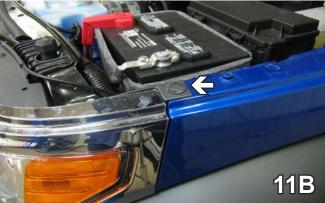
11. **DODGE ONLY:** Remove two pushpins with a flat screwdriver (see photo 11B) and a metric bolt with a 25 torx bit from the top edge of the grille (see photo 11A). Set pushpins and bolt aside to be reinstalled later. Do this to both sides of the vehicle.
