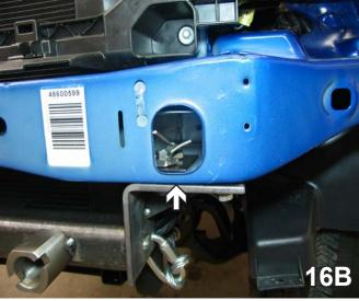
16. BOTH VEHICLES: Align the baseplate with the two existing holes in the bottom of the frame, insert backing plate and 3/8-16 nut plates into the opening on the end of the frame rail to align with these existing holes. Some vehicles may need to have these existing holes reamed with the 13/32" drill bit to acquire the proper fit. Tighten the 3/8-16x2" hex bolts, 3/8" flat washers and 3/8" lock washers with the 9/16" socket. Do this to both sides of the vehicle.
