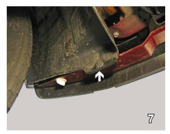
JEEP ONLY: Underneath the front fascia, using a flat screwdriver remove the plastic push pin. Do this to both sides of the vehicle.
