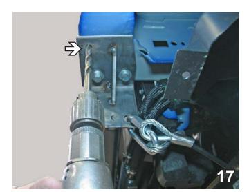
17. BOTH VEHICLES: Using the baseplate as a template, drill a hole into the frame rail with the 13/32" drill bit. Insert the 3/8-16 nut plate into the opening on the back side of the frame support to align with the drilled hole, tighten the 3/8-16 1 1/2" hex bolt and 3/8" lock washer with the 9/16" socket. Do this to both sides of the vehicle.
