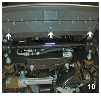
10. **DODGE ONLY:** Using a flat screwdriver, remove three pushpins from underneath the bumper. Set pushpins aside to be reinstalled later.
