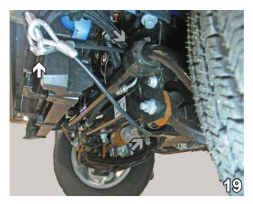
19. BOTH VEHICLES: Attach the permanent baseplate safety cables to the provided convenience link on the baseplate. The photo above shows the recommended installation of the cables to frame of vehicle. Additional options may interfere with suggested mounting; in this case, secure the cables to a solid piece of the frame as described in the General Information sheet. Be sure the safety cables do not rub against any hoses or moving parts. Do this on BOTH sides of the vehicle.
