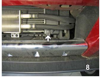
8. **JEEP ONLY:** Using a flat screwdriver in front remove two more push pins, one on each side. (Some models may have three pushpins.) Pull fascia corners out to the side and then forward to release. Set fascia aside carefully to be reinstalled later. (JEEP: Go to Step 14)
