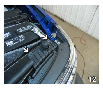
12. DODGE ONLY: Using a 25 torx bit, remove two metric bolts right in front of the battery (see white arrow). Then remove a metric bolt located in the corner, from both sides of the vehicle (see grey arrow). Set bolts aside to be reinstalled later.
