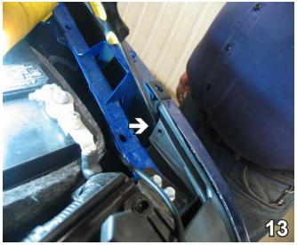
13. DODGE ONLY: Using a flat screwdriver, pull plastic forward to loosen. Do this to both sides of the vehicle. The bumper and grille can then be removed and carefully set aside to be reinstalled later.
