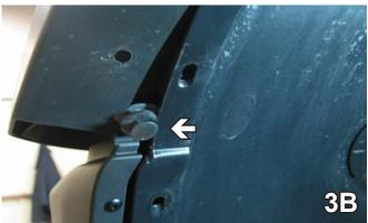
3. DODGE ONLY: Using a diagonal cutters, cut off pop rivet located above the top pushpin (see photo 3A). Then pull plastic back to locate and remove pushpin. The pop rivet will be replaced with a new one from the bolt bag and the pushpin will be set aside to be reinstalled later. Do this to both sides of the vehicle.
