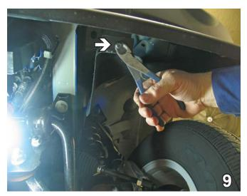
DODGE ONLY: Using a diagonal cutters, remove the pop rivet from the plastic skid pan underneath bumper. New pop rivets found in the bolt bag, will be installed later. Do this to both sides of the vehicle.
