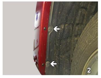
2. **JEEP ONLY:** Remove three push pins and lower two pop rivets with the flat screwdriver and side cutters. Do this to both sides of the vehicle.
