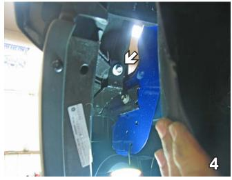
4. BOTH VEHICLES: After removing the pop rivet and pushpin, pull plastic back far enough to reach the top silver bolt. Using a 10MM socket, remove bolt and set aside to be reinstalled later. Do this to both sides of the vehicle.
