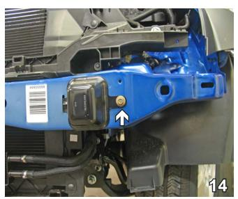
14. BOTH VEHICLES: Remove the metric bolt from the bumper hub with a 10MM socket. Set hub and bolt aside to be reinstalled later. Do this to both sides of the vehicle.
