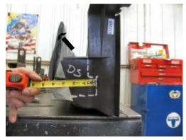
**12.** Measure and mark 6 1/4" and 8 1/4" down from the top edge of the air dam on the driver's side. Draw a line from front edge of air dam (Black arrow in photo on the right) down to the 6 1/4", mark toward the back of air dam 3/4" and down to 6 1/2" mark and then mark a line to the front of vehicle. Remove this front area from the air dam with the utility knife (White arrow in photo to the left).
