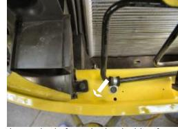
Remove the push pin from the back side of metal bumper, on both sides, remove air dam and set aside.
