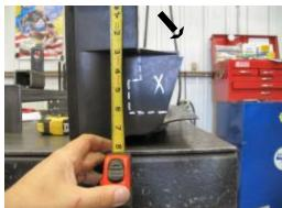
11. Measure and mark 4 1/2" and 6 1/2" down from the top edge of the air dam on the passenger's side. Draw a line from front edge of air dam (Black arrow in photo above) down to the 4 1/2",
