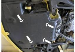
**5.** Remove the four metric bolts from the belly pan using the 8MM socket, release the two clips on the sides of belly pan, set aside.
