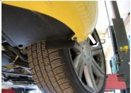
**3.** Just forward of front tire is a Torx screw. Remove with the 30 Torx socket, on both sides.
