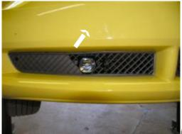
**14.** Reinstall fascia (Left photo above). Be sure that all of the electrical components are plugged in properly. With fascia install complete, hold lower grill section as close to its original position as possible and cut opening in lower grill to allow attachment tab receiver and convenience link (Safety cable connection point) to come through the lower grill. Reinstall lower grill (Right photo above).
