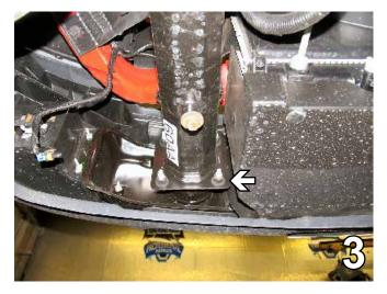
Using the 18MM socket, remove four metric nuts. Located just behind the metal bumper, on the frame end. Set the metric nuts aside to be reinstalled later. Pull the metal bumper forward, unplug the electrical connections and set the metal bumper aside to be reinstalled later.
