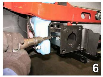
Using the baseplate as a template, drill the remaining three holes with the 17/32" drill bit. Do this to both sides of the vehicle.
