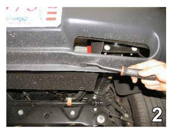
2. Remove the pushpin from the lower edge of the fascia just below the license plate. Set the pushpin aside to be reinstalled later. Do this to both sides of the vehicle.
