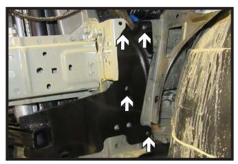
20. On the driver side of the vehicle start drilling the four (4) 3/8" holes need for the bracket. Start with the top two (2) holes, then drill the bottom hole, and finally drill the middle hole. Make sure the bracket stays level while drilling each hole.
