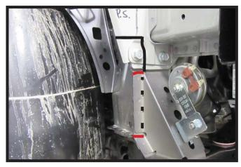
13. On the passenger side use a reciprocating saw to cut along the marked area (black) across and down. Then make two (2) slots (red) as indicated. Using a hammer bend the piece forward along the dotted line.
