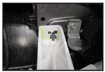
26. When reattaching the windshield wiper fluid reservoir slot out the top hole using a drill bit as indicated so that the reservoir does not hit the baseplate. Then use a 6MM x 30 bolt with a flat washer when reattaching the bottom of the reservoir. Reconnect fluid lines.
