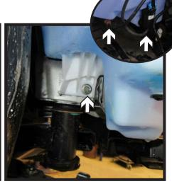
10. Remove the one (1) push pin from the top of the windshield wiper fluid reservoir. Using a 10MM socket, remove the one (1) bolt from the upper front of the reservoir, and the one (1) bolt on the back side of the reservoir. Unplug the two (2) connections from the front of the reservoir, plug the fluid lines, and remove the reservoir.
