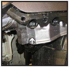
9. Using a 10MM socket, remove four (4) bolts, with two (2) on top, one (1) below, and one (1) on the side. Disconnect the wiring, remove headlights and set aside. Do this for both sides of the vehicle.
