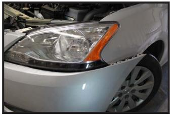
7. Pull the corners of the fascia away from the vehicle disconnecting any electrical connections and set the fascia aside.
