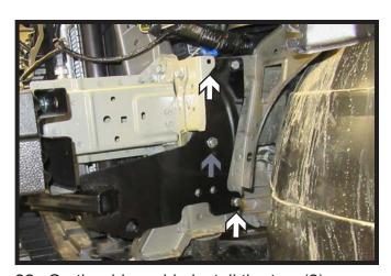
22. On the driver side install the two (2) remaining 3/8"-16 x 1-1/4" Hex Head bolts with a flat washer and nylon lock nut on the back as indicated (white). Then insert one (1) 3/8"-16 x 1-1/2" Hex Head bolt and a Whiz nut with 14" wire on the back (gray).
