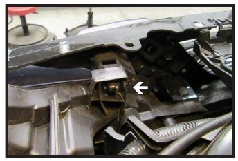
Using a flat screwdriver, push in the pictured clip, and pop the plastic piece out. Do this for both sides of the vehicle.
