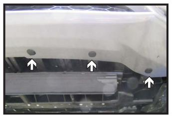
5. Using 10MM socket, underneath the fascia, remove three (3) bolts. Next, remove three (3) push pins. Do this for both sides of the vehicle.
