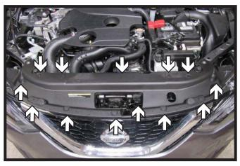
1. Remove thirteen (13) push pins from the fascia cover. Remove fascia cover and set aside.
