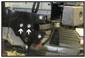
23. On the passenger side install the remaining two (2) 3/8" x 1-1/4" bolts with nylon lock nuts on the back.
