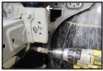
21. On the driver side start a 3/8"-16 x 1-1/4" Hex Head bolt with the flat washer and nylon lock nut on the back in one (1) of the top drilled holes. Then using a 1" hole saw drill out the center access hole, do this on both sides of the vehicle.
