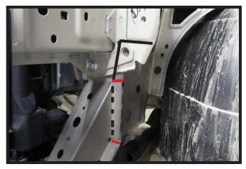
14. On the driver side use a reciprocating saw to cut along the marked area (black) across and down. Then make two (2) slots (red) as indicated Use a hammer to bend the piece forward along the dotted line.
