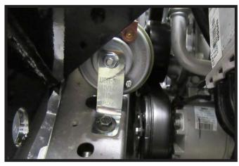
25. Bend the horn bracket to allow for baseplate clearance and reattach the horn as indicated.
