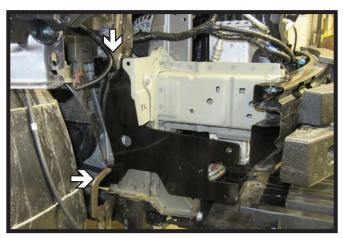
16. Slide on the passenger side plate so that it is level at the top of the frame and flush with the bottom back piece as indicated. Use vice grip to hold into place.
