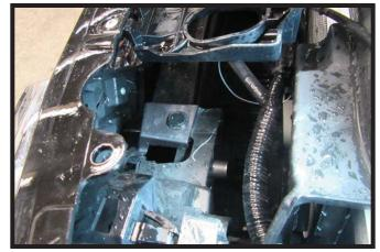
Remove the push pin from the inner fascia. Do this for both sides of the vehicle.
